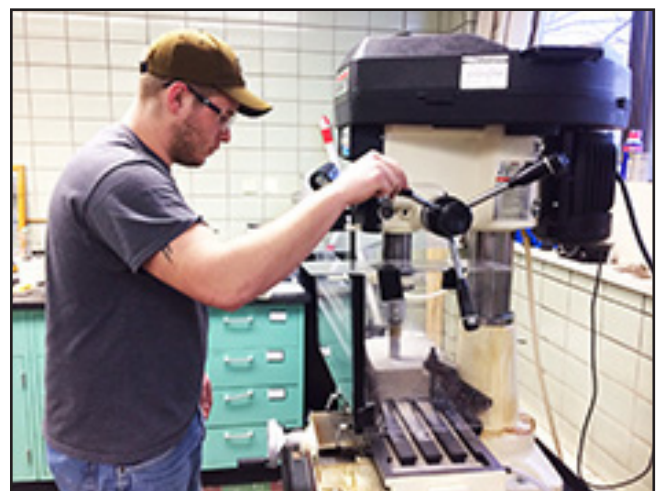
Grad Student Nick Wander coring Indiana Limestone for rock mechanics experiments. The rock was collected from the facade of Zook Hall during renovation last year.
